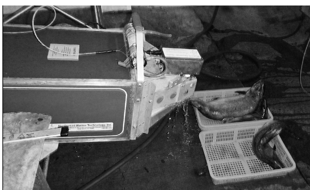
Figure 2. Northwest Marine Technology R9500 tunnel detector with the optional diverter gate for automated sorting of untagged and potentially coded-wire tagged fish. The tunnel detector was installed at a fish processing plant in Kodiak, Alaska.
