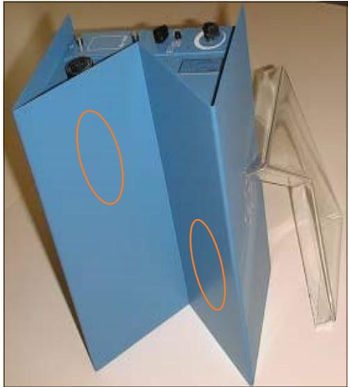
1. The V-Detector is sensitive to movement and will beep if jostled or bumped. To avoid this, position it on a firm surface. The V-Detector can be mounted on a post or wall using the two  $\frac{1}{4}$ " x 20 threaded sockets on the rear panel. Do not force long mounting screws into the rear panel mounting sockets. The sockets are closed to prevent water entry.
