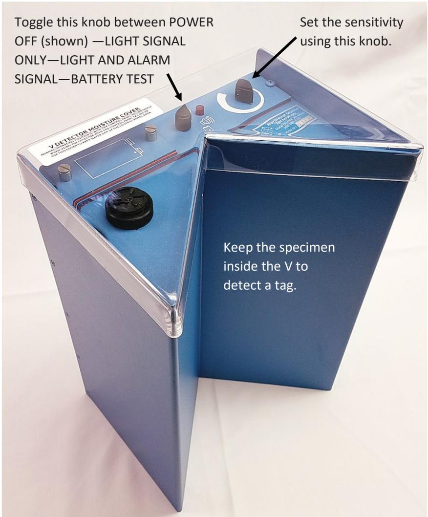
2. Turn the selector knob to the battery check position. If the detector beeps and the light comes on, the battery is satisfactory. If not, install a fresh battery.
