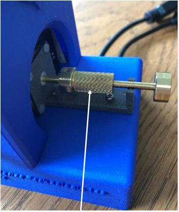
Insert the pencil into the tag viewer so that it rests in the cradle. Roll your finger back and forth on the handle to smoothly rotate the tag.
