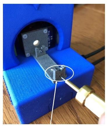
Pick up a tag with the tag pencil. The tag should be sticking straight out from the tip. If not, touch the tag to the magnet on the end of the cradle to straighten it.
