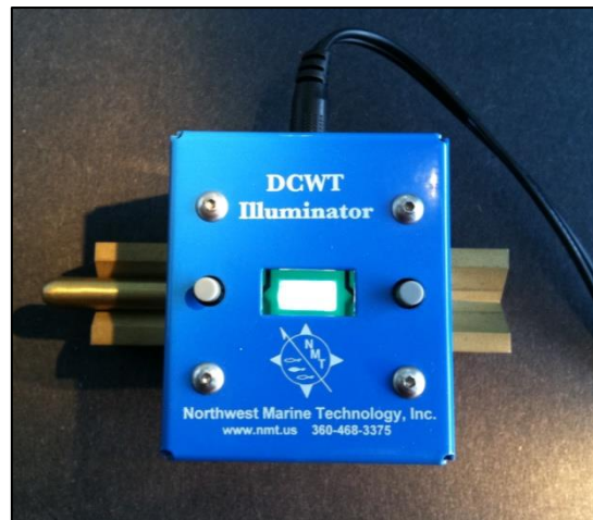
Figure 24 A tag reading jig (top) and Illuminator (bottom) facilitate reading CWT with a microscope. The brass pencils in the tag reading jig holds the tag so that the tag can be rotated during reading.
