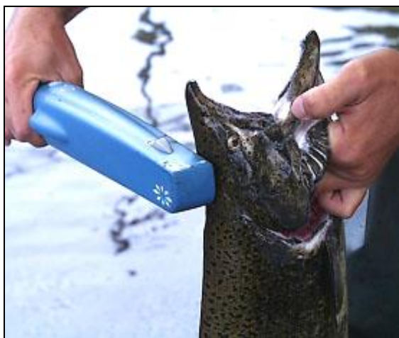
Figure 14 Blue Wand Detector being used to detect a tag in a Chinook Salmon.
