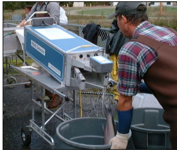
Figure 18 R8000 Tunnel Detector with a diverter gate to separate tagged and untagged adult salmon returning to Marblemount Hatchery, WA. A tagged fish has just passed through and is going into the left bin.
