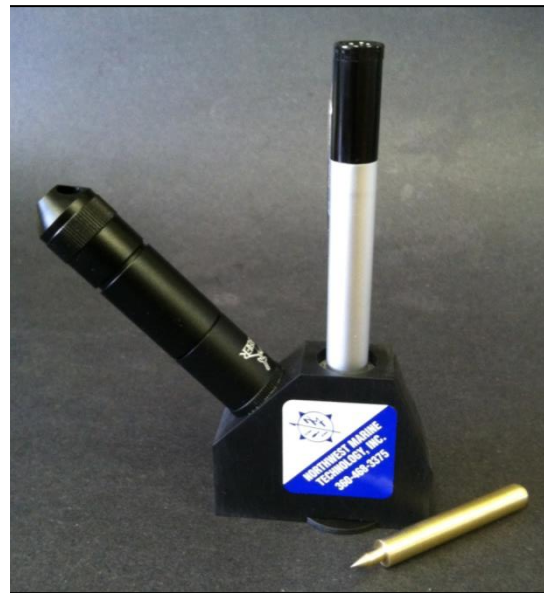
Figure 23 The Magniviewer is a portable, battery-operated device used to magnify and view CWT. Individual tags can be held with the brass pencil and viewed in the Magniviewer, or a strand of CWT wire can be inserted into it. The Magniviewer operates on AA batteries and can be used anywhere.
