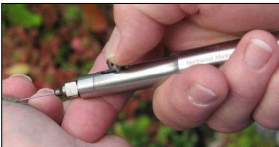
Figure 9 Single Shot Tag Injector for injecting precut sequential CWT.
