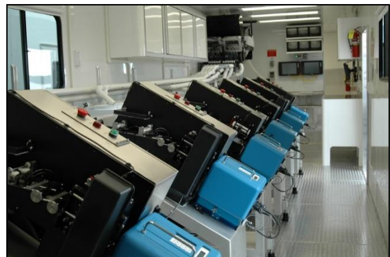
Figure 10 AutoFish System is contained in a mobile trailer (top) that can be moved between hatcheries. The interior (bottom) has a holding tank for fish waiting to be processed, a sorter that measures and sorts fish into size categories, and marking and tagging lines for injection of CWT and adipose fin clipping.
