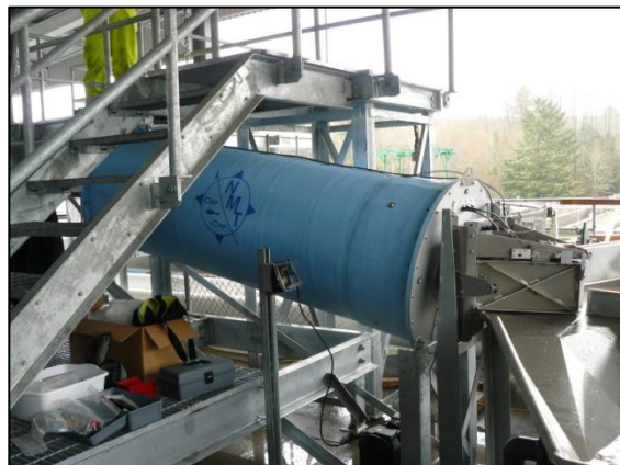
Figure 19 This T13 Detector is permanently installed at Cowlitz Hatchery in Washington and includes a gate for
