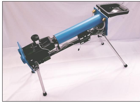
Figure 20: Quality Control Device (QCD) in use connected to a Mark IV.
