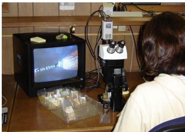
Figure 7. A recovered CWT, magnified and displayed on a monitor for easy reading (Photo provided by ODFW).
