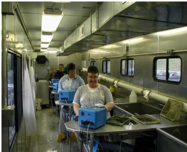
Figure 3. Interior of a manual tagging trailer using Mark IV tag injectors (Photograph by George Nandor).
