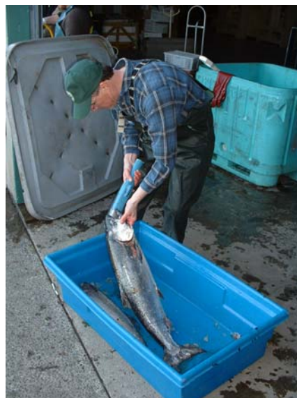
Figure 5. Electronic sampling of commercially caught Chinook salmon using a handheld wand detector (Photo by George Nandor).
