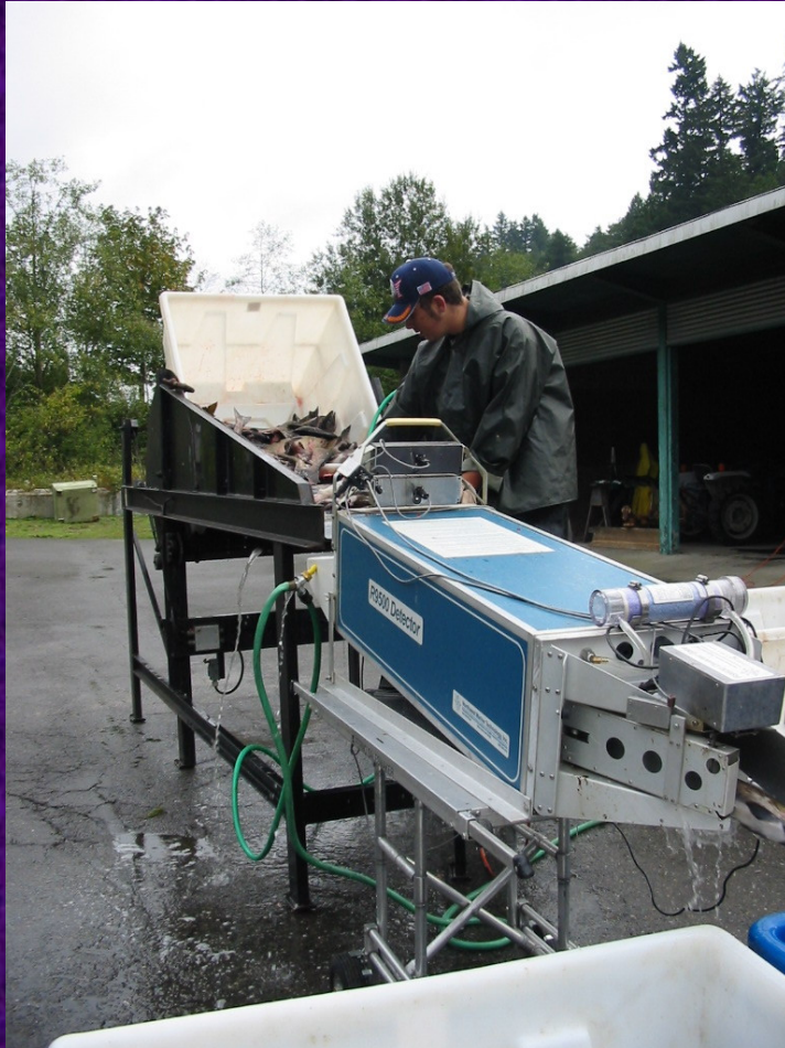
Wand and tube CWT detectors
